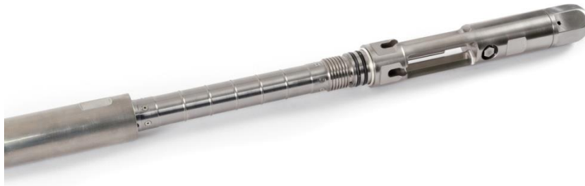
Figure 45 - Expose the memory module and leave the tool to cool down
