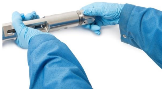
Figure 13 - Attaching the bullnose to the memory module
