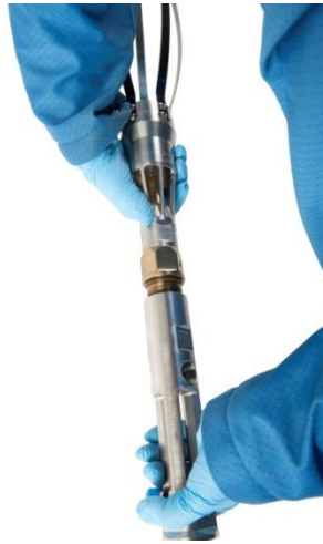
Figure 11 - Hand tighten the centralizer in place
