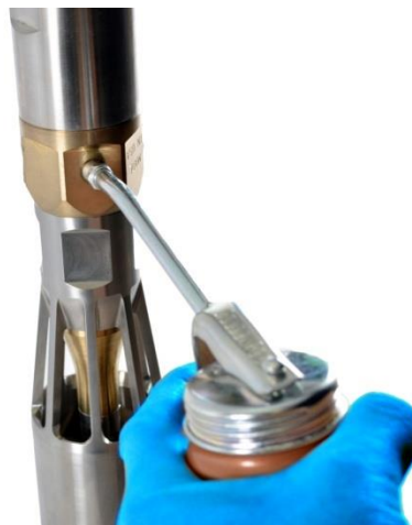
Figure 39 - Filling the spinner with oil
