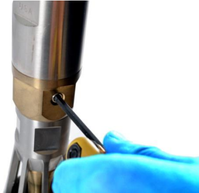
Figure 38 - Removing the oil plugs from the spinner
