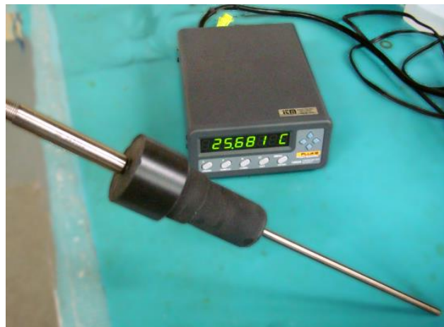
Figure 1 - RTD thermometer and heat insulator for testing
