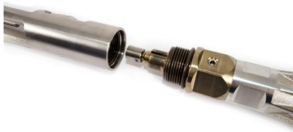
Figure 6 - Insert the spinner into the memory module
