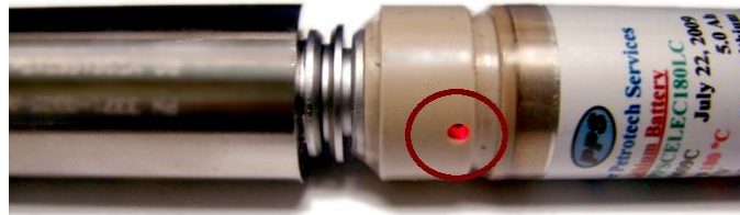
Figure 35 - Attaching the battery to the module
