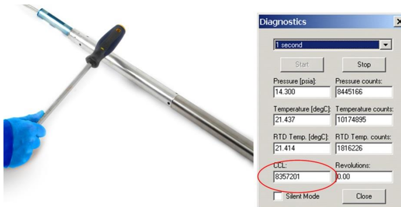
Figure 27 - Testing CCL to check the reading in Diagnostics panel
