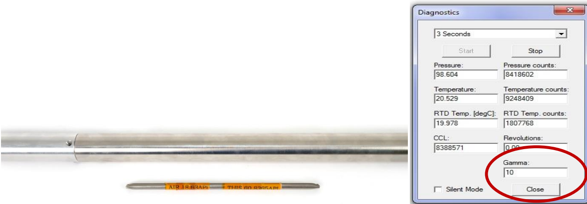
Figure 30 - Checking gamma with gamma ray tester beside the module
