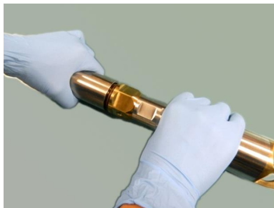
Figure 7 - Hand screw the spinner onto the pressure sub
