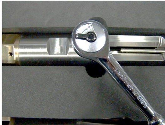
Figure 51 - Installing the pressure filter with a socket wrench
