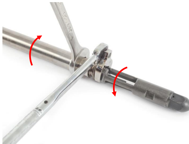
Figure 41 - Correct wrench positions to remove the housing
