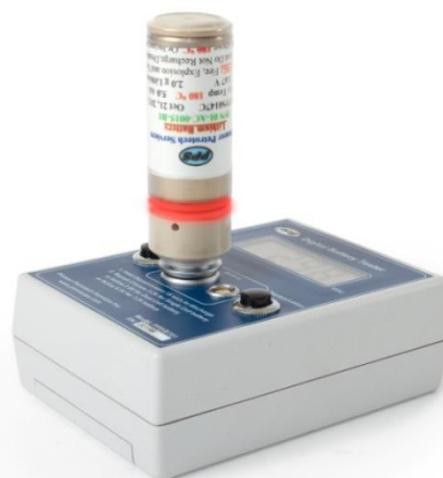
Figure 34 - Plugging the battery into the PPS battery tester
