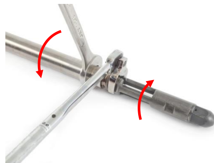
Figure 36 - Steps for installing the housing on the memory module (1.75" OD)
